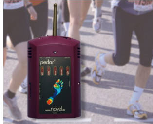
Dynamic pressure measuring between foot and shoe
