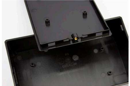
Multiple PCB mounting points in the base and lid (sizes 1 & 2 have two mounting points in the lid and four in the base, sizes 3 and 4 have four mounting points in the lid and base), with minimal screws required.
